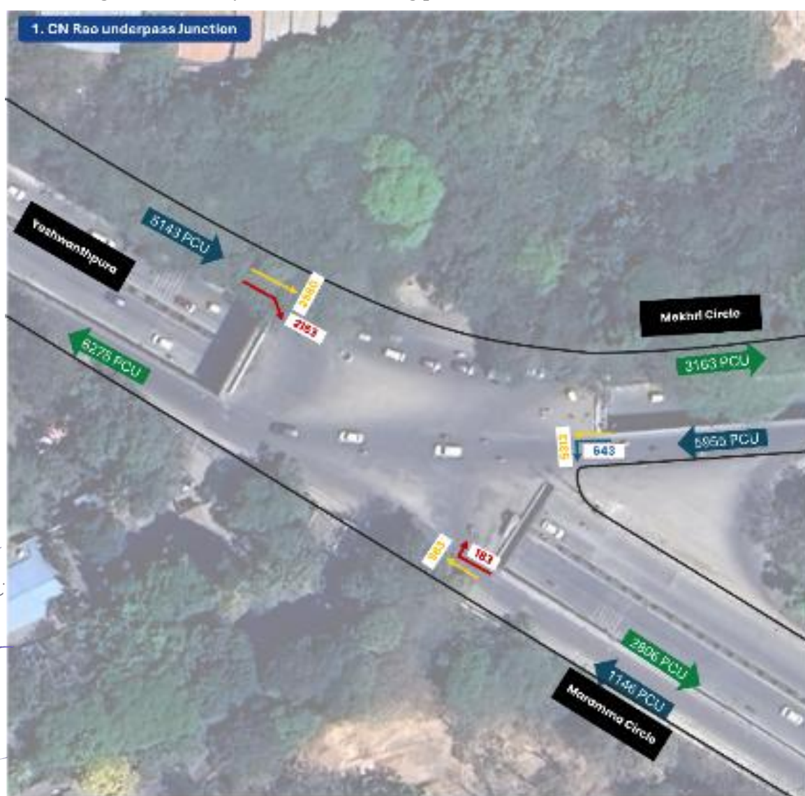
Figure 95: TMC at CN Rao Underpass Junction
