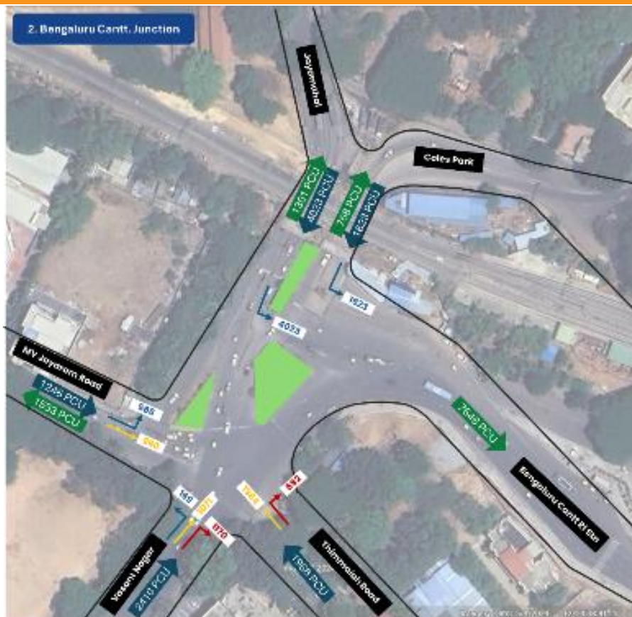
Figure 96: TMC at Bengaluru Cantt Junction
